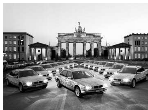
Figure 1: Fleet of BMW 750 hL (liquid H 2 -powered vehicles).
